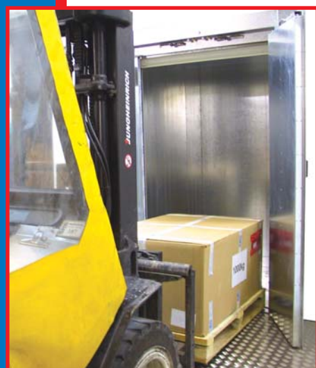
Highest safety standard, each cabin with electronic overload device
